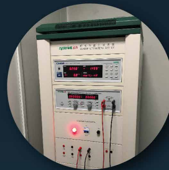
Control system (Measurement Station, Power Supply, Photometer)
